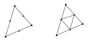
If the triangle is subdivided, the process is then repeated on each of the four subtriangles. Eventually, the triangles will be small enough to adequately approximate the surface.
