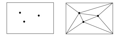
The corner vertices of the database area are included, so that the entire space is triangularized. The case of three point targets produced eight triangles in the triangularization shown. The triangularization is not unique.
